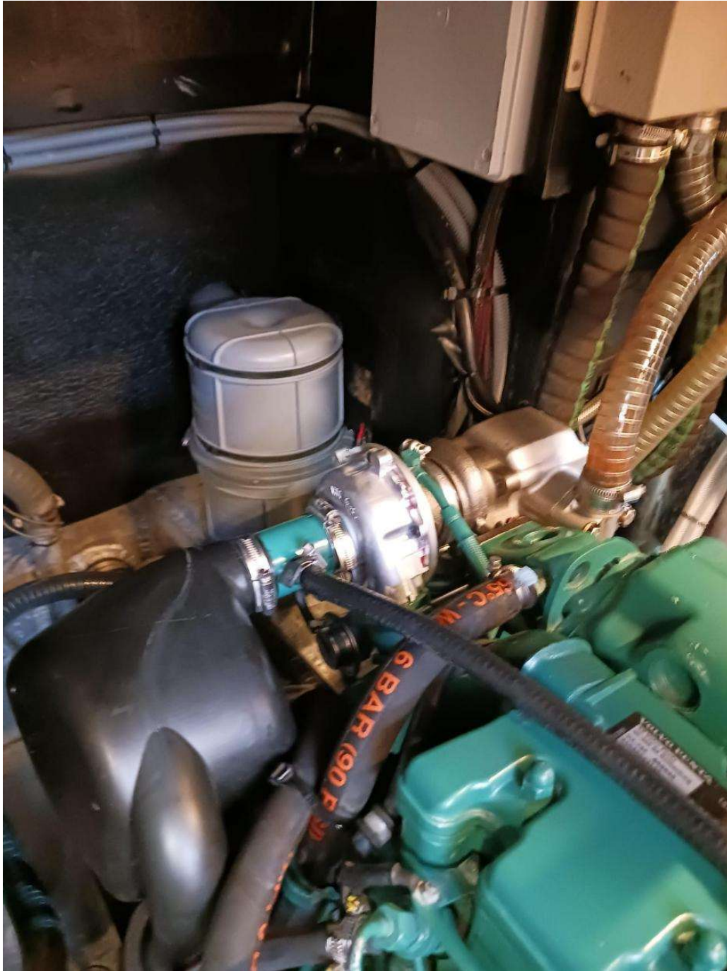
Spiffy New Turbo Mounted on the Engine. Note the Inox Exhaust Elbow.
