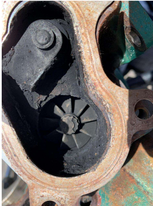
Outer Chamber of the Turbo After the Turbine and the Turbine. Note the heavy Corrosion near the Turbine which Impedes its Rotation a Little.
