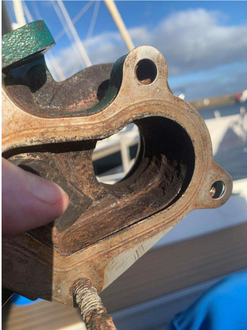
Turbo Exhaust outer Chamber before the Turbine 3. Heavy Corrosion Burr where the Turbine lets the Hot Gaz into the Elbow.
