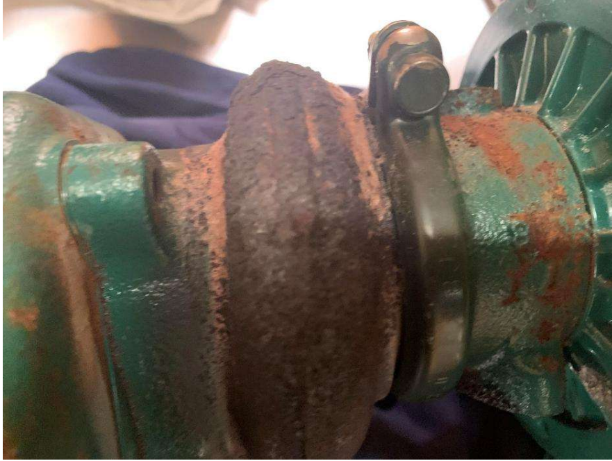
Rust Bucket Turbo Housing on the Hot Side.
